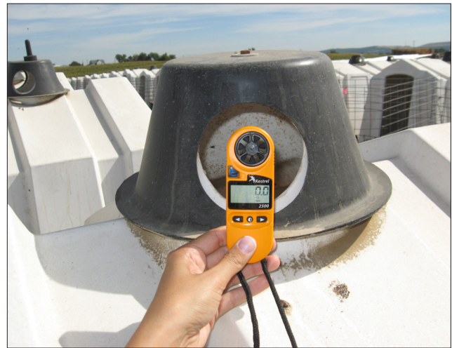
Figure 25. Anemometer measuring airflow through the ridge vent of a plastic hutch.
