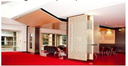
Extensive use of glass partitions enables deep daylight penetration and access to outside views to more than 90% of regularly occupied and seated floor spaces. A 29% reduction in lighting power density below ASHRAE requirements was achieved with high efficiency lighting and zoned controls.
