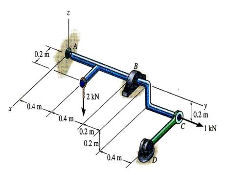
Given: A rod is supported by a ball-and-socket joint at A, a journal bearing at B and a short link at C
