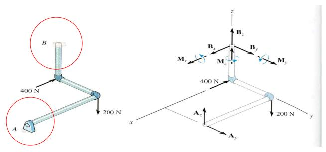
Redundant Constraints: When a body has more supports than necessary to hold it in equilibrium, it becomes statically indeterminate.
