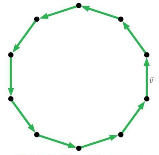
The lengths of the velocity vectors are the same, indicating constant speed, but the direction of each vector is different. This is a changing velocity.
