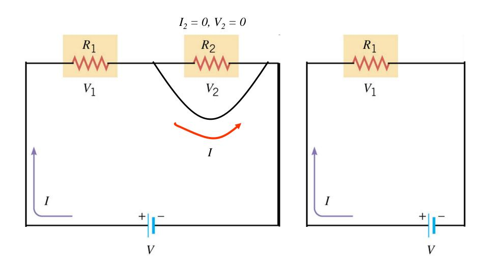
A resistor(s) in a branch is shorted if you can go from one node/junction on one side to the other side by a route that has no resistors or batteries.
