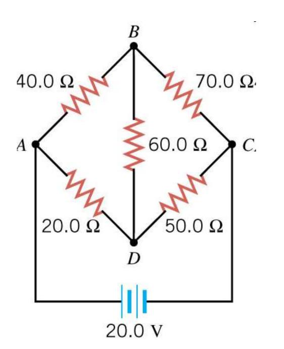
Circuit with no series or parallel resistors.
