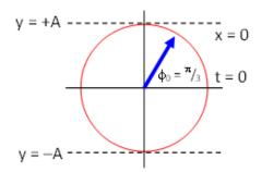
The snapshot graph, a plot of y versus x, for t=0 can be sketched by referring to the phasor or reference circle diagram. The y-component of the amplitude is positive at x=0,  $y=A\sin(\pi/3)=0.866A$ . As x increases, the phase  $0.55x-62.8t+\pi/3$  also increases and the vector rotates counter clockwise to maximum y amplitude A. The snapshot graph therefore looks like:
