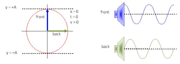
Clearly, the two waveforms will line up peak to peak, i.e. interfere constructively, when the back speaker is moved back  $\frac{1}{4}\lambda$  or d = 0.375 m.
