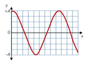
The history graph, a plot of y versus t, for x = 0 can be sketched by referring to the phasor or reference circle diagram. The y-component of the amplitude is maximum, A. As t increases, the phase  $8.38x + 126t + \pi$  also increases and the vector rotates counter clockwise to zero amplitude. The history graph therefore looks like identical to the snapshot graph:
