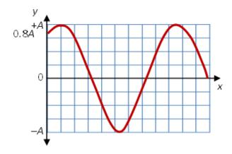
The vector in the phasor diagram rotates clockwise with increasing t in the y versus t, or history graph if the wave is moving to the right as it does here. So here the y starts at 0.8A and falls to equilibrium, zero amplitude. The history graph looks like.
