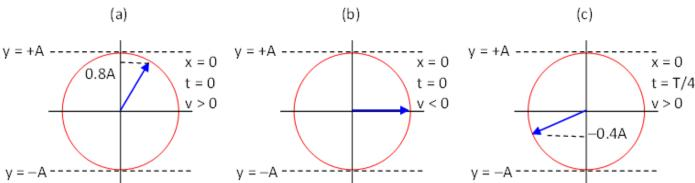
(a) The phase constant  $\varphi_0$  is the angle measured counter clockwise from the positive *x*-axis to the vector when the diagram shows x = 0 and t = 0. Simple trigonometry indicates that  $\varphi_0 = \arcsin(0.8) = 53.1^{\circ}$  or 0.927 rad.
