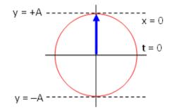
The snapshot graph, a plot of y versus x, for t = 0 can be sketched by referring to the phasor or reference circle diagram. The y-component of the amplitude is maximum, A. As x increases, the phase  $8.38x + 126t + \pi$  also increases and the vector rotates counter clockwise to zero amplitude. The snapshot graph therefore looks like:
