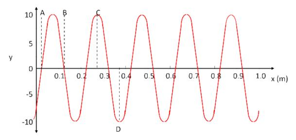
The phase constant  $\varphi_0$  is the angle measured counter clockwise from the positive x-axis to the vector when the phasor diagram shows x = 0 and t = 0. The snapshot graph above shows that the initial amplitude is -7.5 or -0.75A where A = 10. The graph next has zero amplitude. Since the vector in a phasor diagram moves counter clockwise with increasing x, the vector must be in the fourth quadrant as shown in the diagram below.
