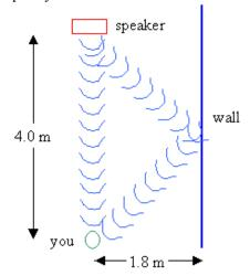
The speed of sound is 340 m/s. The lowest sound intensity occurs for destructive interference. If the wall is flexible, when the sound reflects the wave will not change phase. Thus the condition for destructive inference is
