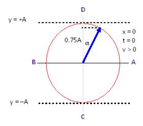
We can find the angle  $\alpha$  in the phasor diagram,  $\alpha = \arccos(0.75) = 41.41^{\circ}$  or  $0.7227 \ rad$ . The phase constant is therefore  $\varphi_0 = 90^{\circ} - \alpha = 48.59^{\circ} = 0.8481 \ rad$ .
