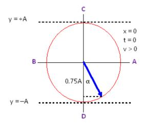
We can find the angle  $\alpha$  in the phasor diagram,  $\alpha = \arccos(0.75) = 41.41^{\circ}$  or  $0.7227 \ rad$ . The phase constant is therefore  $\varphi_0 = \alpha + 270^{\circ} = 311.41^{\circ} = 5.435 \ rad$ .
