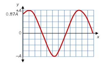
The history graph, a plot of y versus t, for x=0 can be sketched by referring to the phasor or reference circle diagram. The y-component of the amplitude is positive at t=0,  $y=A\sin(\pi/3)=0.866A$ . As t increases, the phase  $0.55x-62.8t+\pi/3$  decreases and the vector rotates clockwise to zero amplitude. The history graph therefore looks like:
