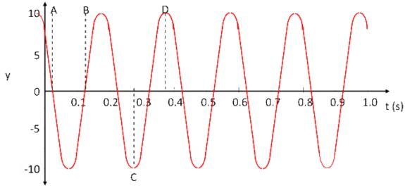
The phase constant  $\varphi_0$  is the angle measured counter clockwise from the positive x-axis to the vector when the phasor diagram shows x = 0 and t = 0. The history graph above shows that the initial amplitude is 7.5 or 0.75A where A = 10. The graph next has zero amplitude. Since the vector in a phasor diagram moves clockwise with increasing t for a wave travelling to the right, the vector must be in the first quadrant as shown in the diagram below.
