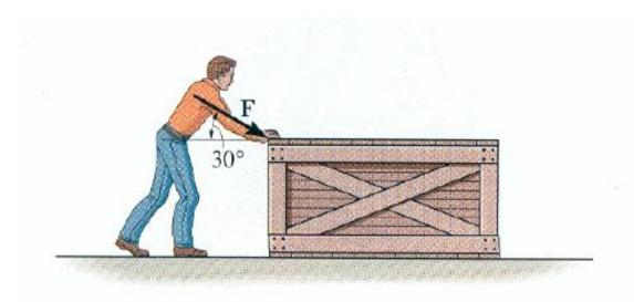
If a man is pushing a 100 lb crate, how large a force F must he exert to start moving the crate?
