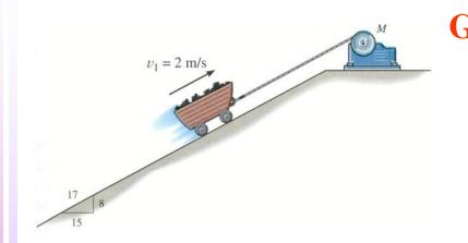
Given: The 400 kg mine car is hoisted up the incline. The force in the cable is  $F = (3200t^2) \text{ N}$ . The car has an initial velocity of  $v_i = 2 \text{ m/s}$  at t = 0.
