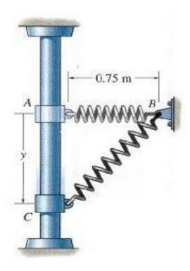
**Given:** The mass of the collar is 2 kg and the spring constant is 60 N/m. The collar has no velocity at A and the spring is un-deformed at A.
