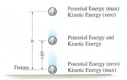
When a ball of weight W is dropped (from rest) from a height h above the ground, the potential energy stored in the ball is converted to kinetic energy as the ball drops.
