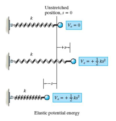
V<sub>e</sub> (where 'e' denotes an elastic spring) has the distance "s" raised to a power (the result of an integration) or
