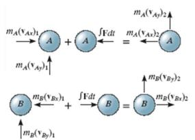
Conservation of momentum and the coefficient of restitution equation are applied along the line of impact (x-axis):
