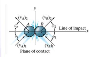
In an oblique impact, one or both of the particles' motion is at an angle to the line of impact. Typically, there will be four unknowns: the magnitudes and directions of the final velocities.
