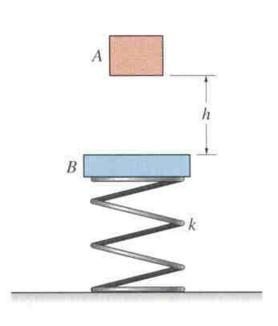
Given: A 2 kg block A is released from rest, falls a distance h = 0.5 m, and strikes plate B (3 kg mass). The coefficient of restitution between A and B is e = 0.6, and the spring stiffness is k = 30 N/m.
