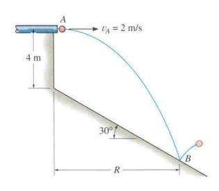
Given: A 0.5 kg ball is ejected from the tube at A with a horizontal velocity  $v_A = 2$  m/s. The coefficient of restitution at B is e = 0.6.
