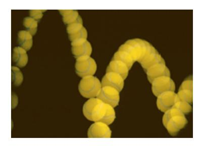
The quality of a tennis ball is measured by the height of its bounce. This can be quantified by the coefficient of restitution of the ball.
