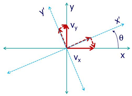
$$\begin{aligned} v_x' &= v_x \cos\theta + v_y \sin\theta \\ v_y' &= -v_x \sin\theta + v_y \cos\theta \end{aligned} \qquad \begin{pmatrix} v_x' \\ v_y' \end{pmatrix} = \begin{pmatrix} \cos\theta & \sin\theta \\ -\sin\theta & \cos\theta \end{pmatrix} \begin{pmatrix} v_x \\ v_y \end{pmatrix}$$
