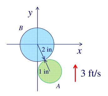
Given: Disk A weighs 2 lb and is moving at 3 ft/s. Disk B weighs 11 lb and is initially at rest. The coefficient of restitution is e = 0.6.
