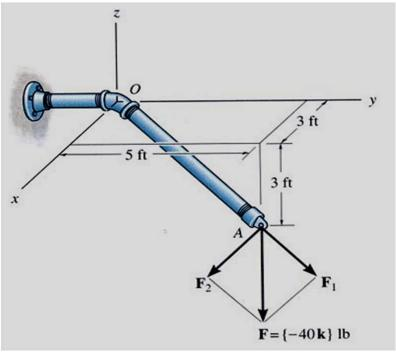
For force F at Point A, what component of it  $(F_1)$  acts along the pipe OA? What component  $(F_2)$  acts perpendicular to the pipe?
