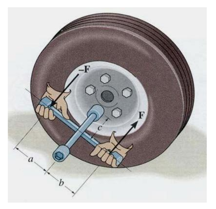
The crossbar lug wrench is being used to loosen a lug net. What is the effect of changing dimensions a, b, or c on the force that must be applied?
