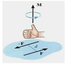
A couple is defined as two parallel forces with the same magnitude but opposite in direction separated by a perpendicular distance d.
