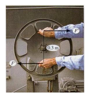
A torque or moment of  $12 \text{ N} \cdot \text{m}$  is required to rotate the wheel. Which one of the two grips of the wheel above will require less force to rotate the wheel?
