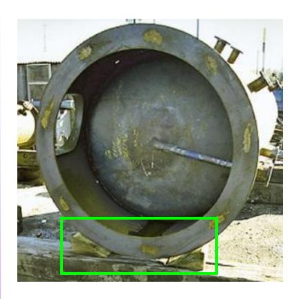
Wedges are used to adjust the elevation or provide stability for heavy objects such as this large steel vessel.
