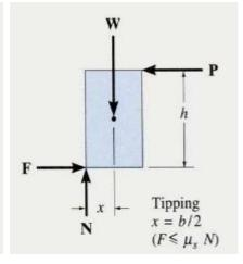
For a given W and h, how can we determine if the block will slide first or tip first? In this case, we have four unknowns (F, N, x, and P) and only three E-of-E.
