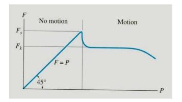
The <u>maximum friction force</u> is attained just before the block begins to move (a situation that is called "impending motion"). The value of the force is found using  $F_s = \mu_s \ N$ , where  $\mu_s$  is called the coefficient of static friction. The value of  $\mu_s$  depends on the materials in contact.
