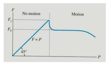
To study the characteristics of the friction force F, let us assume that tipping does not occur (i.e., "h" is small or "a" is large). Then we gradually increase the magnitude of the force P. Typically, experiments show that the friction force F varies with P, as shown in the right figure above.
