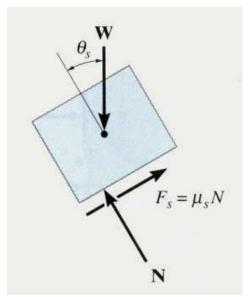
A block with weight w is placed on an inclined plane. The plane is slowly tilted until the block just begins to slip.
