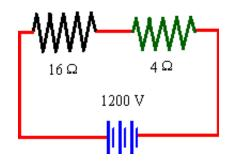
Finally, we note that the 4  $\Omega$  and 16  $\Omega$  resistor are in series and may be replaced by a single 20  $\Omega$  resistor as shown below.
