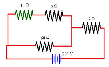
Next the  $10~\Omega$  and  $2~\Omega$  resistor are in series. Since  $10~\Omega + 2~\Omega = 12~\Omega$ , we replace these two resistors by a single  $12~\Omega$  resistor.
