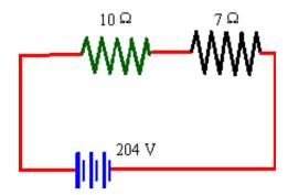
Finally, we note that the  $10 \Omega$  and  $7 \Omega$  resistor are in series and may be replaced by a single  $17 \Omega$  resistor as shown below.
