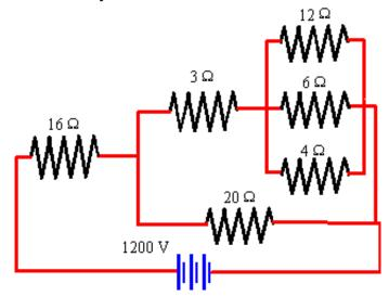
We reduce circuits which are a combination of series and parallel resistors piece by piece. Examining the circuit we see that the 12  $\Omega$ , 6  $\Omega$ , and 4  $\Omega$  resistor are in parallel. Since 1/12 + 1/6 + 1/4 = 6/12, these resistors may be replace by a single 2  $\Omega$  resistor, as shown below.
