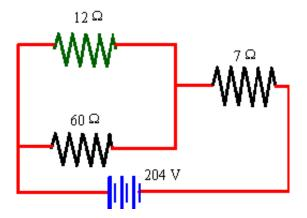
Next we observe that the 12  $\Omega$  and 60  $\Omega$  resistors are in parallel. Since 1/12 + 1/60 = 6/60, these resistors may be replace by a single 10  $\Omega$ resistor, as shown below.
