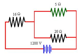
Next we observe that the 5  $\Omega$  and 20  $\Omega$  resistors are in parallel. Since 1/5 + 1/20 = 5/20, these resistors may be replace by a single 4  $\Omega$  resistor, as shown below.
