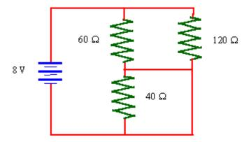
The 40  $\Omega$  resistor is in parallel with just a wire of zero resistance - that is it is being short-circuited. The two arms may be replaced by a single wire since
