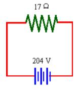
The equivalent resistance is thus 17  $\Omega$ . It has a voltage drop of 204 V. Using Ohm's Law, it carries a current  $I_{17} = V/R = 204 \text{ V} / 17 \Omega = 12 \text{ A}$ . It dissipates a power of  $P_{17} = V^2/R = 2448 \text{ W}$ .
