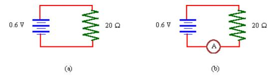
For diagram (a) we just use Ohm's law to determine the current
