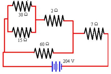
We reduce circuits which are a combination of series and parallel resistors piece by piece. Examining the circuit we see that the 30  $\Omega$  and 15  $\Omega$  resistor are in parallel. Since 1/30 + 1/15 = 1/10, these resistors may be replace by a single  $10 \Omega$  resistor, as shown below.
