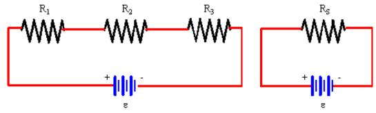
(i) Since there are no nodes or branches between the three resistors, the three resistors are in series. For series resistors, the equivalent resistance is
