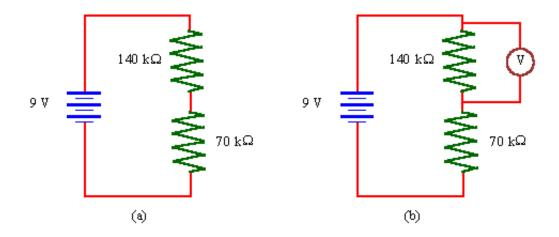
For diagram (a) we can determine the potential difference over the 140 k $\Omega$  resistor quite simply. It is twice as big as the 70 k $\Omega$  resistor. Hence it uses twice as much energy and so has twice the potential difference. That is it gets  $2/3 \times 9$  Volts = 6 Volts.
