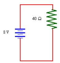
Thus the equivalent resistance of the circuit is  $40~\Omega$ . The current from the battery is  $I = V/R = (8~V)/(40~\Omega) = 0.20~A$ . The equivalent resistor is actually the  $60~\Omega$  resistor and the  $120~\Omega$  resistor connected in parallel, so they all have the same potential difference of 8~V. The  $60~\Omega$  being twice as small as the  $120~\Omega$  resistor gets  $^2/_3^P$  of the current, 0.133~A, while the  $120~\Omega$  resistor the rest, 0.067~A.
