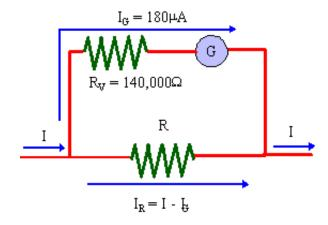
Since the voltmeter is parallel with the resistor, the voltage drop across both is the same. The voltage drop across the coil is
