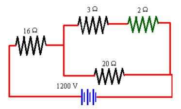
Next the 2  $\Omega$  and 3  $\Omega$  resistor are in series. Since 2  $\Omega$  + 3  $\Omega$  = 5  $\Omega$  , we replace these two resistors by a single 5  $\Omega$  resistor.
