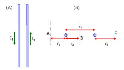
The magnetic field is tangential to the cross-section of a wire. The direction is clockwise or counterclockwise using a Right Hand Rule. To use the Right Hand Rule, you curl your hand around the wire with your thumb pointing in the direction of the current. The magnetic field "circulates" in the same direction that your hand is curling.
