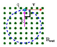
The magnetic force is  $F = qvBsin(90^\circ) = qvB$ . It is directed to the centre of the circle, so it is the centripetal force. Applying Newton's Second Law
