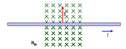
Only the portion of the wire in the magnetic field experience the force. The magnitude of the magnetic force is given by  $F = ILBsin(\theta)$ . Here,
