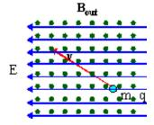
The forces acting on the charge are its weight, mg, the Coulomb force,  $F_C = qE$ , and the magnetic force,  $F_m = qvBsin(\theta)$ . Since the charge is positive, the Coulomb force point to the left along the electric field. Using the Right Hand Rule, the magnetic force is in the plane of the paper and perpendicular to the particle's velocity, so  $\theta = 90^\circ$ . Furthermore, some geometry indicates that the magnetic force makes a  $50^\circ$  angle to the positive x axis.
