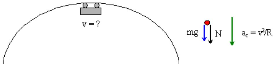
Applying Newton's Second Law,  $F_y = ma_y$ , we get  $-N - mg = -mv^2/R$ . The car loses contact when  $N = 0$ , so our equation for the speed at which the car leaves the track becomes  $v = [gR]^{1/2} = [9.81 \times 150]^{1/2} = 38.4 \text{ m/s} = 138 \text{ km/h}$ . If the car goes faster than this speed, it will remain safely in contact with the track.
