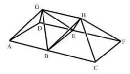
You will need to use the techniques of vector mechanics to express each force as a Cartesian vector and apply the equations of equilibrium. Then you will solve for the tensile and compressive forces in each member.
