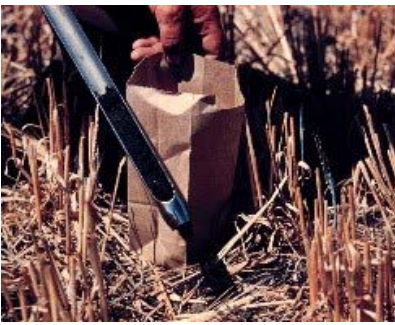
Figure 5. Sampling using a hand-held soil probe to 6 inches.
