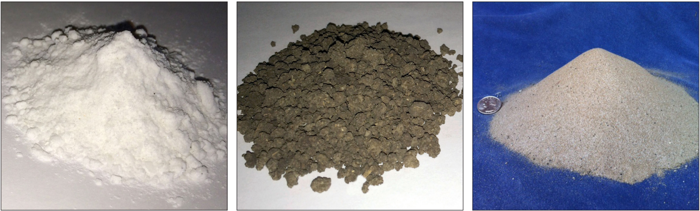
Figure 4. Nutrient recovery products including (left to right) bio-ammonium sulfate crystals, phosphorus-rich solids, and phosphorus containing struvite crystals. Photos of ammonium sulfate crystals and solids courtesy of Craig Frear. Photo of struvite crystals courtesy of Keith Bowers.
